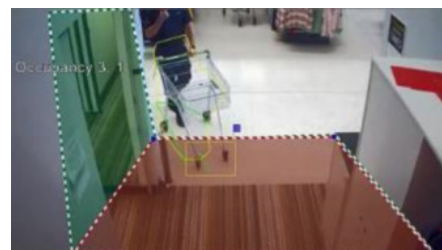
Figure 6: Modern video analytics based on direction detection, data gathering and occupancy monitoring to help retailers to maintain social distance in their shops
