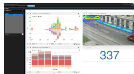
Figure 2: Occupancy and heat mapping in Xprotect Smart Client
