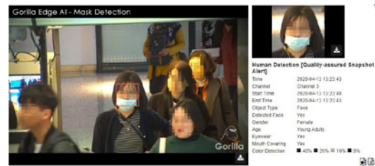
Figure 15: Face metadata in XProtect Smart Client detecting real time: Eyewear: YES, Mask: YES
