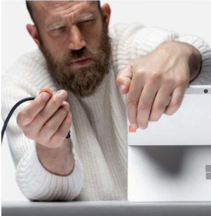
Left Image: Joshua using port indicators to hold a USB cable and laptop USB port. Right Image: A person using opener support to pull a laptop kickstand open.
