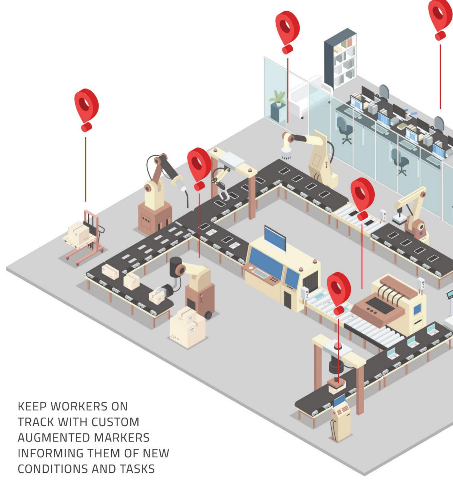
Remote users can place AR knowledge markers in the field, or the operations manager can insert them from the AVR web portal. These markers can be annotated with IoT data, text, voice, video, 3D data, and other media. AR Assist is designed to enable hands-free collaboration and traceability between individual workers and large institutions.
