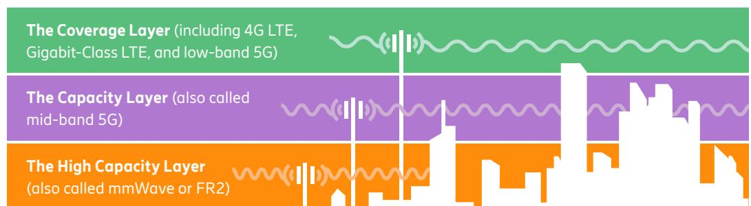
The combination of the coverage and capacity layer has also been called "Sub-6 GHz" or FR1.
